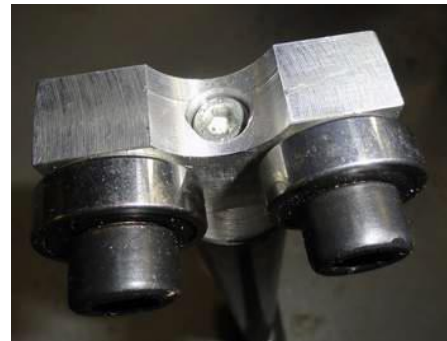
Ball bearings at the end of each arm
