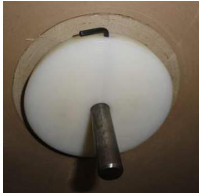
Two rilsan flanges with a steel axle and a clamping screw
