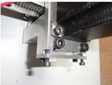
Driving by a toothed gear and a rack and pinion
